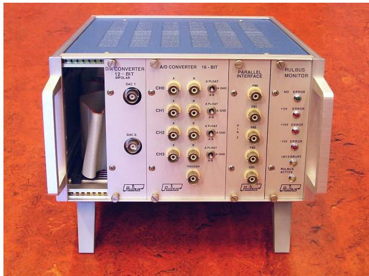
Figure 2.1: A Rulbus rack (half-width)
